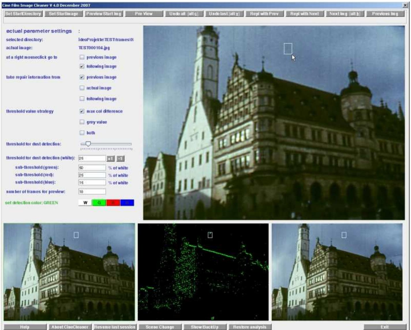
The window has several sections: the control button bars, the message line, the parameter maintenance area and the canvases to present the image to be cleaned, the reference images and the analysis pattern.
