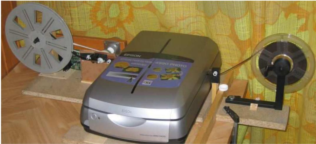
Setup to scan using automated film transport (with Epson 4990 and Pollin stepmotor control)
