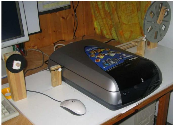
Setup to scan using manual film transport (with Epson 4870)
